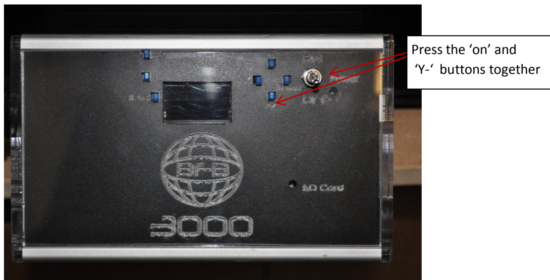
Figure 1: To get to bootloader mode, turn the screen on at the same time as pressing the Y- button.
