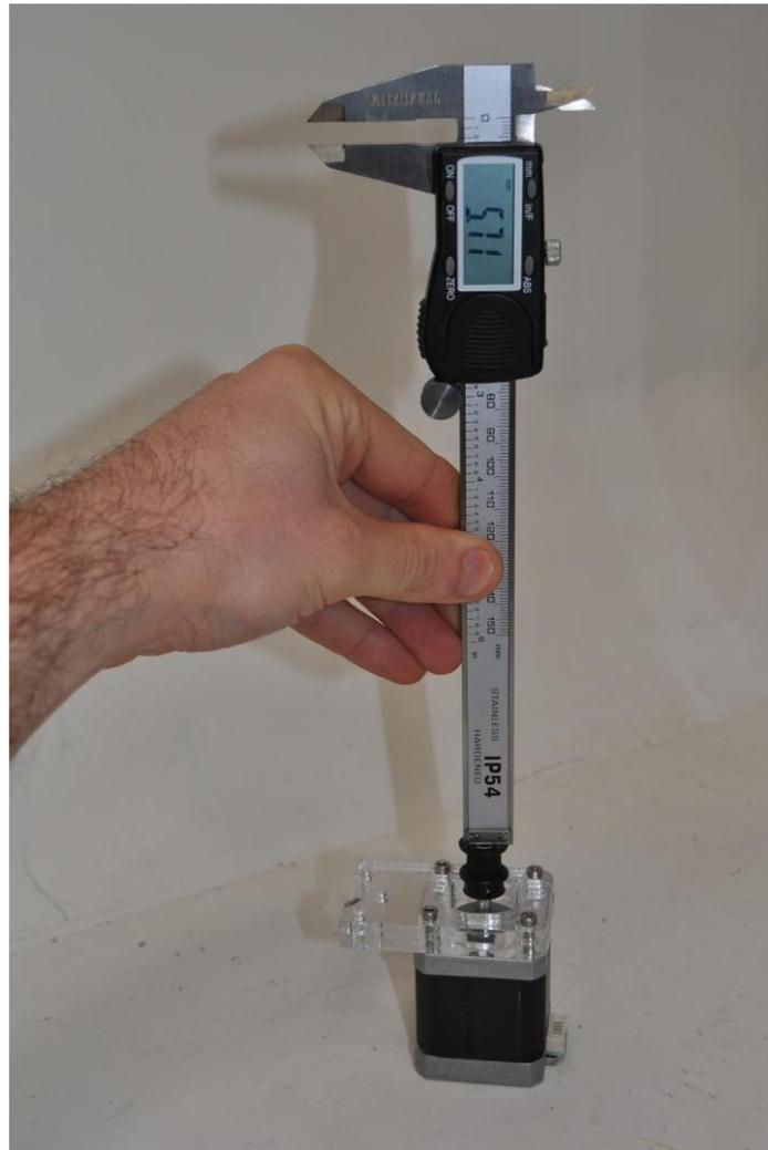
Use the 1.5 mm grub screw to lock the pulley at this position.
