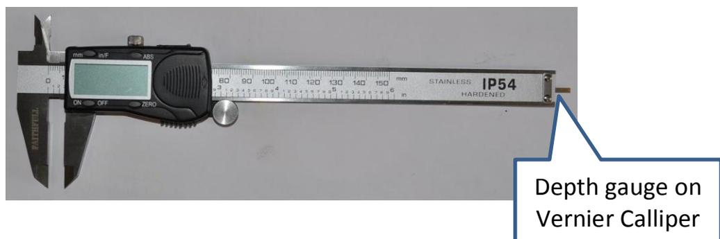
Insert the depth gauge into the top of the pulley and set the height accordingly. Ensure that the bottom of the depth gauge touches the motor shaft, and the end of the callipers sit flush with the top of the motor pulley.
