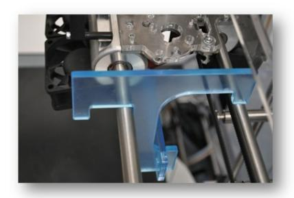
Place the T-pieces across the x axis bars ensuring the parts are, as pictured, resting on the bars not the belt. Place one either side of the X carrage.
