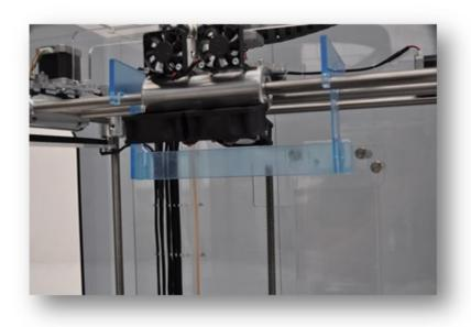
Once your jig is set up as pictured please click here to go to the instructions on how to level the nozzles. Note: the nozzle levelling jig replaces the bed in these instructions.
