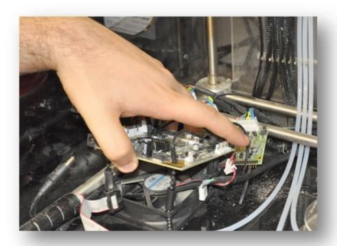
Pull the main controller electronics module from the rubber fasteners.
