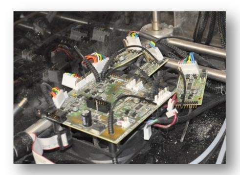
Unplug all looms, ribbon cables and extruder modules from the main controller electronics module.
