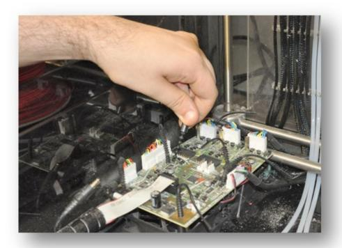
Remove the spacers that are on top of the electronics from the rubber fasteners.
