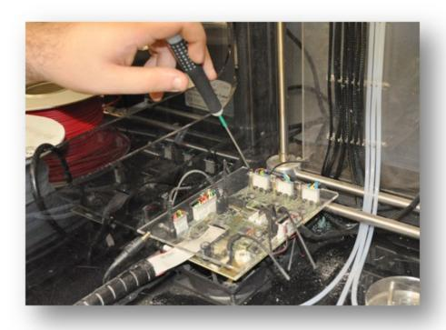
Unscrew the bolts holding the acrylic plate to the extruder modules.
