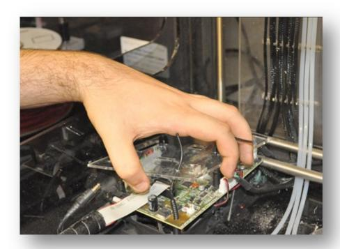
Remove acrylic cover plate by pulling it from the rubber fasteners.
